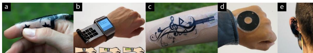
Fig. 29 iSkin : Flexible, Stretchable and Visually Customizable On-Body Touch Sensors for Mobile Computing, Martin Weigel, Tong Lu, Gilles Bailly, Antti Oulasvirta, Carmel Majidi, and Jürgen Steimle, 2015
