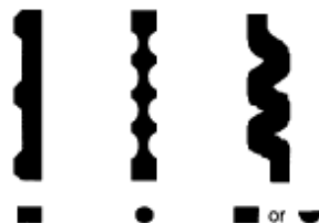
Figure 1. Fibre geometries (from ACI Committee 544, 2002)
