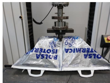
Figure 20. Procedure: (a) System of insulating thermal covering in the sample (b) During the test
