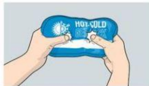
Figure 19. Preparation of the hot conditions: (a) Warm the packs in a microwave set 640W for 30 seconds (b) Knead to distribute the heat evenly (from https://gelpacksdirect.co.uk/pages/how-to-use-a-gel-pack )
