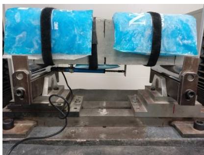
Figure 20. Procedure: (a) System of insulating thermal covering in the sample (b) During the test
