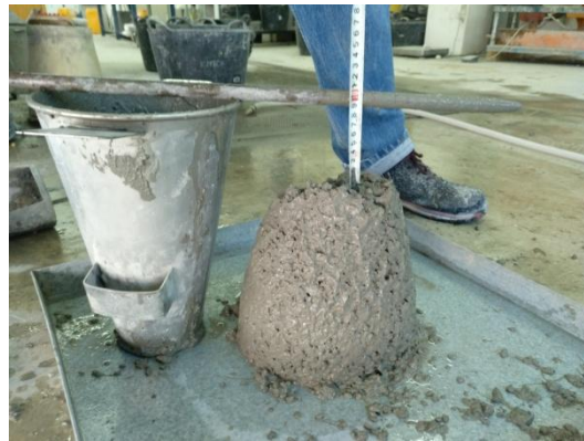
Figure 13. Example of slump test of the Batch 6 S of this study
