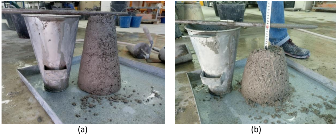
Figure 22. Examples of the visual aspect of the concrete mixes: (a) Batch 6 P2 MFSRC and (b) Batch 6 SFRC.
