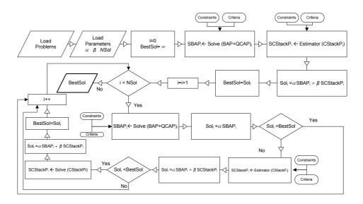
Figure 4.3: Data flow diagram of the Integrated System Functioning.
