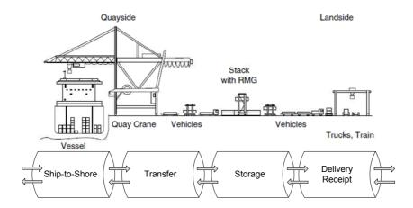
Figure 1.4: Process of unloading and loading a vessel.
