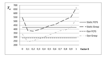
Figure 3.13:  $T_w$  for 20 vessels with sparsely inter-arrival times.
