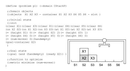
Figure 2.4: Example of problem instance in Container Stacking domain.
