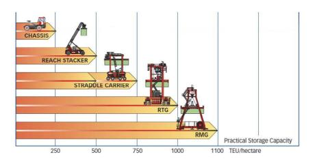
Figure 1.6: Different types of handling equipment and their stacking capacity.
