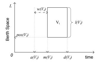
Figure 3.5: Representation of a vessel according its position and times
