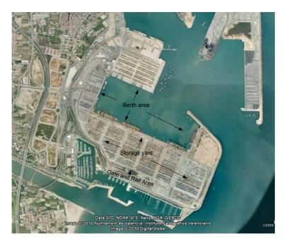
Figure 3.1: Container Terminal at Valencia
