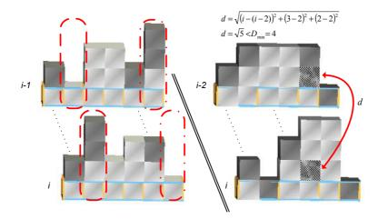
Figure 2.12: (Left) Non-balanced yard-bays. (Right) Proximity of two dangerous containers.
