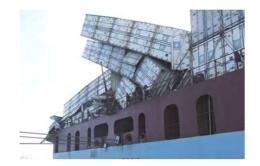
Figure 1.8: Unbalanced yard-bay at one vessel.
