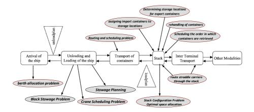
Figure 1.7: Optimization Problems in Container Terminals.
