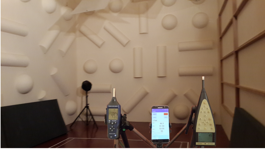
Figure 6.1: Noise calibration using professional devices. Location: reverberant acoustic chamber, at the Universitat Politècnica de València.
