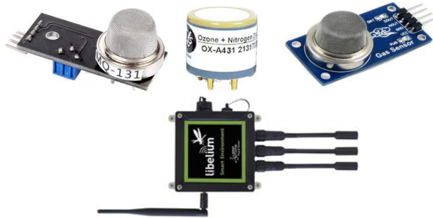
Figure 3.4: Different types of Air Pollution sensors.
