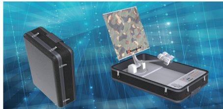
Figure 1.5: The Kuang-Chi flat-panel reflector antenna for Satcom, in a suitcase [18].
