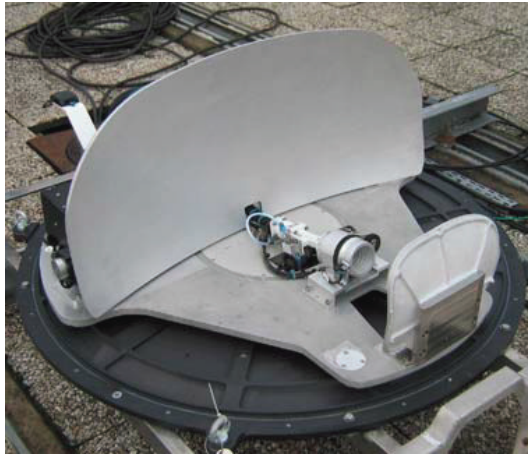
Figure 1.3: Ku-Band dual reflector antenna [16].
