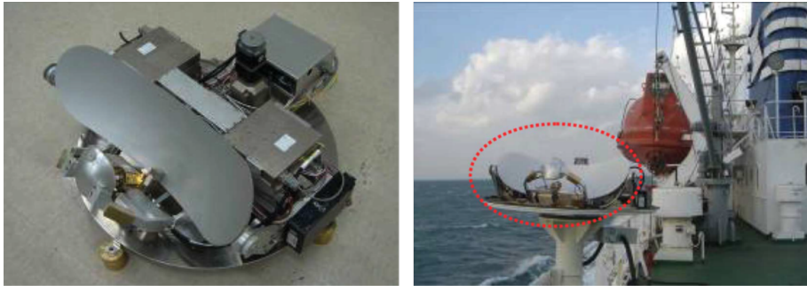
Figure 1.4: (Left) Photo of the entire assembled mobile antenna system and (right) antenna system installed on a large test ship [17].
