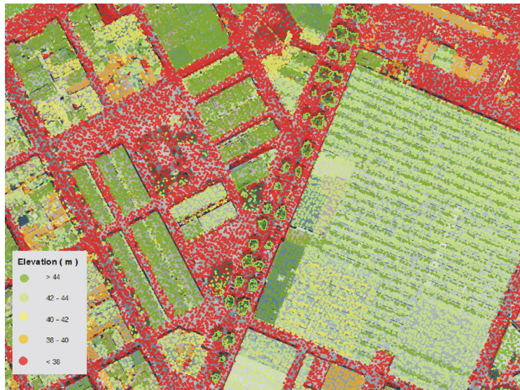
Fig. 4 Includes the distribution of the ALS data used in this study. The perimeters of crown trees extracted from ALS data are in green.
