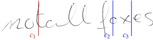
Figure 2.2. Example showing two relevant columns ( c_2 and c_3 ) of the given image and the query keyword “foxes”, and a non-relevant column ( c_1 ). Intuitively, any column of the image belonging to the bounding box of the keyword within the image will be relevant.
