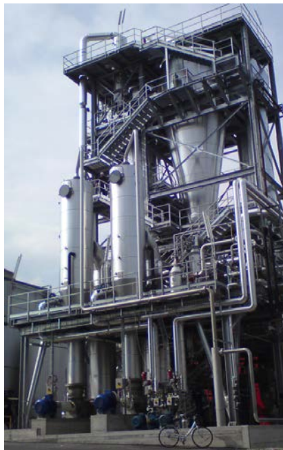
Fig. 2: Schematic of PSSD used for DDGS production
