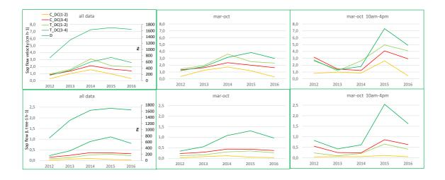
Figure S2. Seasonal mean values of the decoupling coefficient  $\Omega$  in both the control (C) and the cleared (T) plots.
