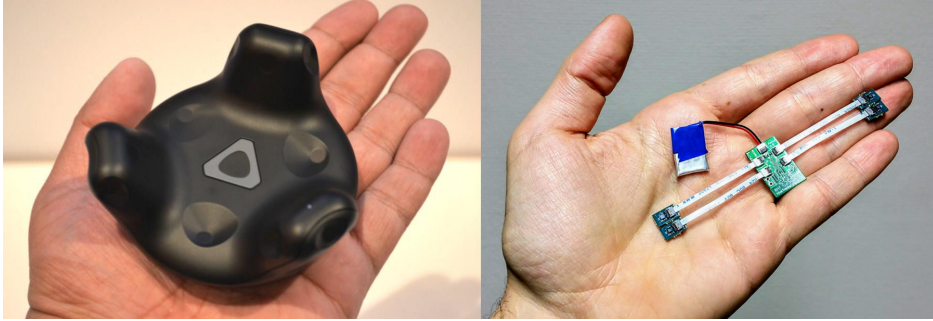
Figure 3.10. Size/weight comparison. Commercial tracker: 10 \times 10 \times 4.2 = 420\text{cm}^3 ; 85g. Hive Tracker: 2.5 \times 1.5 \times 1.1 = 4.13\text{cm}^3 ; 8g.
