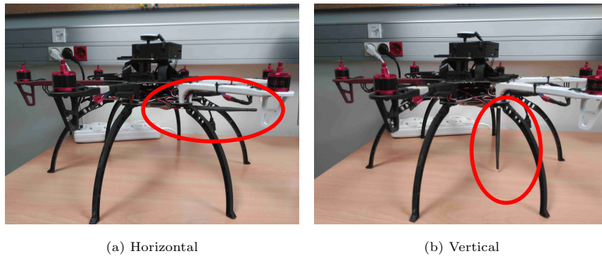
Figure 9: View of the antenna orientation.
