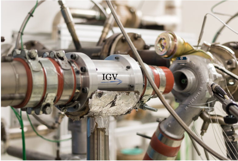
Figure 3.19: IGV integration in turbocharger test bench.
