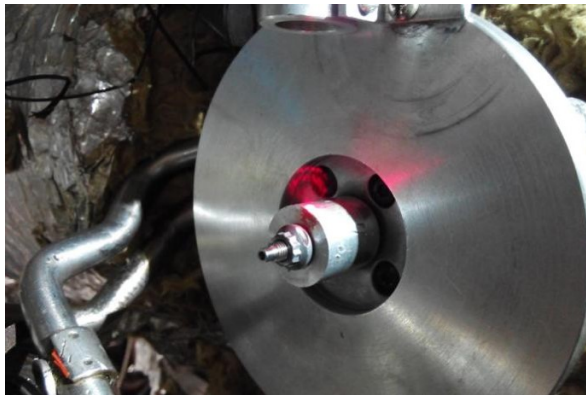
Figure 3.14: Metal cylinder which replaces the compressor wheel
