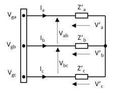
*Fig. 10.* Equivalent circuit with unbalanced star-connected load and without zero-sequence voltage.
