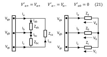
Fig. 9. Original circuit with delta-connected load and its star-connected equivalent.
