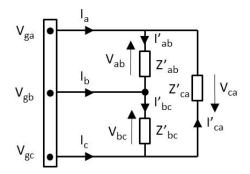
Fig. 8. Equivalent circuit with unbalanced deltaconnected load and without zero-sequence current.
