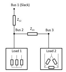
*Fig. 11. Three-wire three-bus electrical system with two unbalanced three-phase linear loads.*
