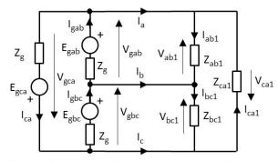
Fig. 6. Three-phase electrical system with deltaconnected generator and delta-connected load.
