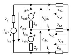
*Fig. 5. Three-phase electrical system with delta-connected generator and star-connected load.*
