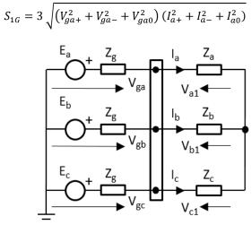
*Fig. 1. Three-phase electrical system with generator and star-connected load.*
