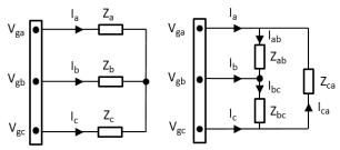
*Fig. 7.* Original circuit with star-connected load and its delta-connected equivalent.
