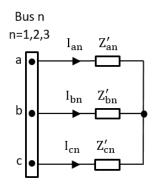
*Fig. 12.* Equivalent circuit 'star-connected' in any of the nodes.
