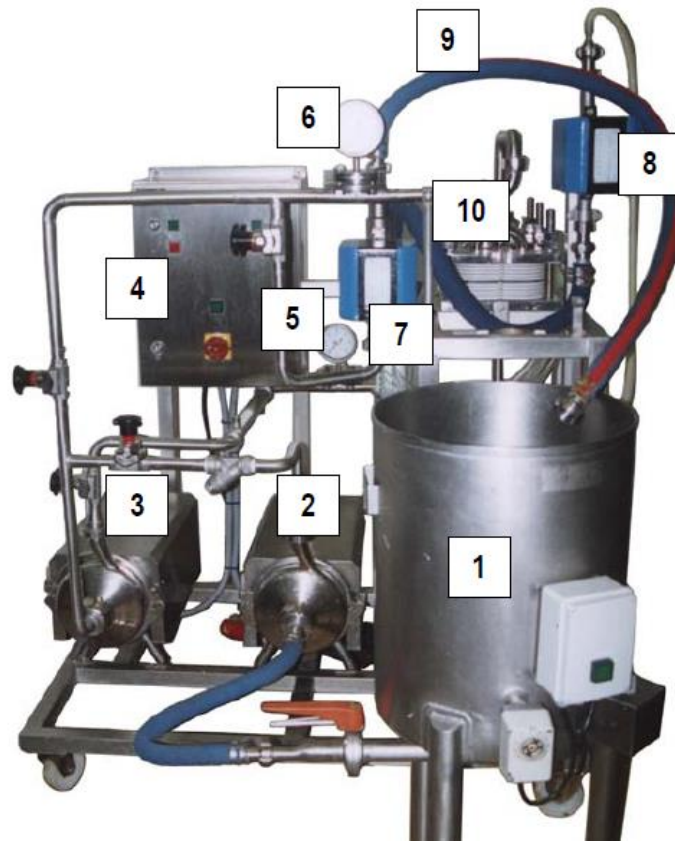
Figure 15. Membrane pilot-plant: (1) Feed tank, 50L, (2) Feed centrifugal pump, (3) Recirculation centrifugal pump, (4) Control panel, (5) Manometer, module entrance, (6) Manometer, module exit, (7) feed flowmeter, (8) permeate flowmeter, (9) thermometer, (10) Membrane exchangeable module type Pleiade UFP 10 BIO.
