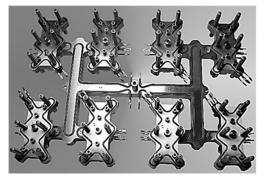
Figure 9: Hot runner system with 48 gates in X-layout [13].
