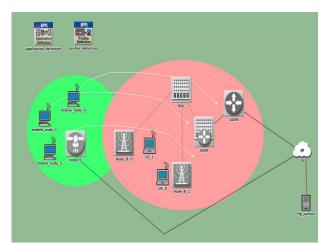
Fig. 2: Simulation topology of handover between WLAN and UMTS
