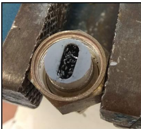
Figure 8.7. Teflon sealing tape and catalyst in the methanation micro reactor.
