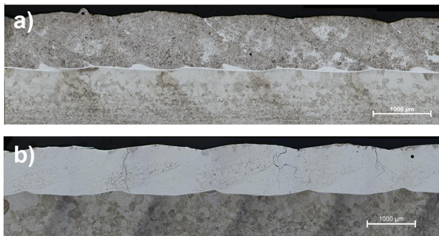
Figure 1. Cross-section of the coatings observed through optical microscopy, a) Coat01 coating ( E = 70 \text{ J/mm}^2 ) and b) Coat04 coating ( E = 180 \text{ J/mm}^2 )
