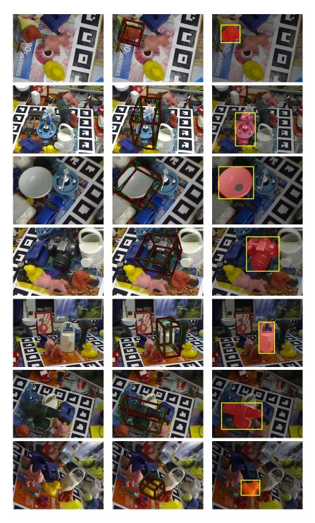
**Figure 7.** Results visualisation of the estimated pose using the LINEMOD dataset. The bounding box projection of the actual pose is shown in red, and the estimated pose by our method is shown in green (best viewed in colour).
