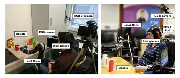
**Figure 1.** AIDE system integrates three different hardware modules: (i) a full-arm robotic exoskeleton or a Jaco2 robot; (ii) multimodal interfaces, consisting of a pair of gaze-tracking glasses (Tobii glasses) and a hybrid brain–computer interface (BCI) based on electroencephalography (EEG) and electrooculography (EOG); and (iii) context recognition sensors: a RGB-D camera to locate the object's pose and a camera to compute the user's head and mouth pose.
