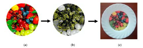
**Figure 4.** Image target: (**a**) Image target; (**b**) Features identified by Vuforia Target Manager; (**c**) Real dish with the image target.
