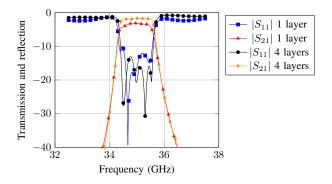
Fig. 5. Comparison between measured results of the typical ESIW single layer filter and the multilayer filter proposed in this paper.
