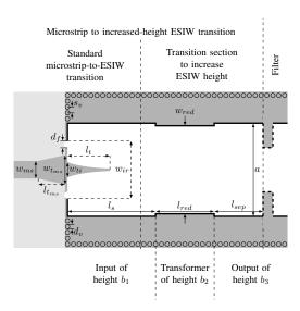
Fig. 1. Proposed microstrip to increased-height ESIW transition that allows the integration of high-performance ESIW filters. Light gray: dielectric substrate. Dark gray: copper metallization on top layer. Black: border metallization used to close the ESIW. White: air.
