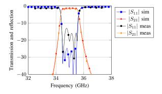
Fig. 4. Comparison between measured and simulated results.
