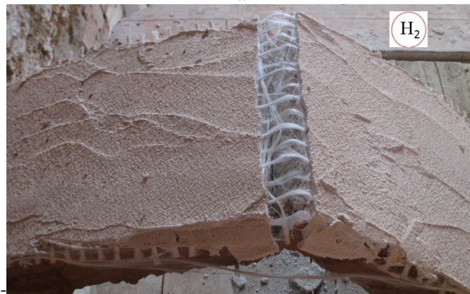
Figure 19: Failure mode of TRM_V. –a: hinges appearance. –b: TRM collapse.
