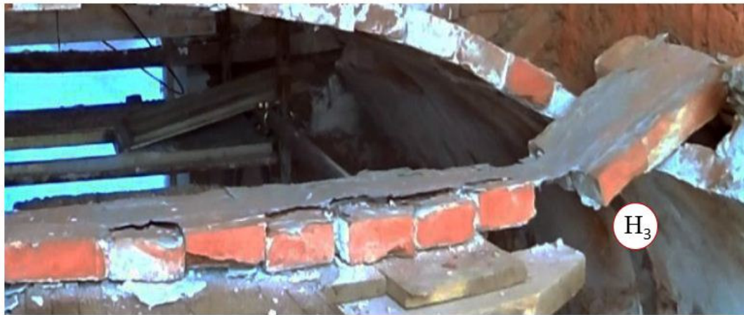
Figure 18: Failure mode for FRP_V –a: Appearance of the first and second hinges. –b: FRP debonding.
