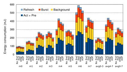
Figure 9: Energy consumption of the prefetching mechanisms.
