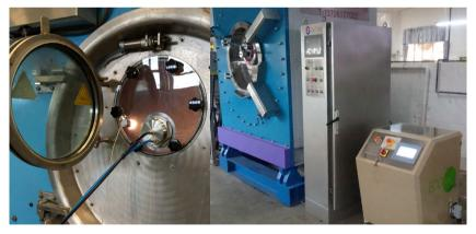
FIGURE 2. ECOFINISH SYSTEM INSTALLED IN THE SYSTEM OF EXHAUSTION IN CONVENTIONAL GARMENT
