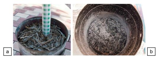
**Figure 9.** Autocombustion container: (**a**) *Arundo donax* leaves and sheath leaves before ignition; (**b**) remaining ashes after autocombustion.
