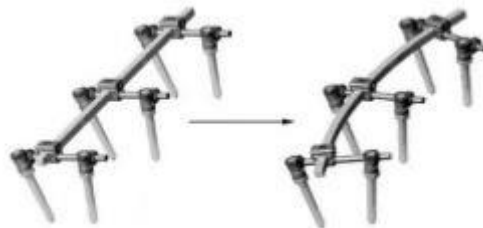
Figure 6 - Spinal rod. The first image shows the straightened rod with anchorage system and the second image shows the original curve of the rod after applying heat [24].
