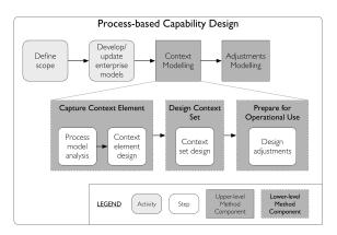
Figure 4: The procedure of the process-based capability design pathway. The particular focus is on Context Modelling upper-level method component, since it defines procedures and provides guidelines to identify variability in business process models
