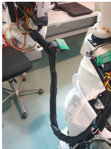
Figure 38. Final cable cover
