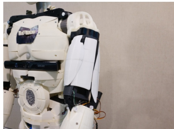
Figure 30. Bicep after repairing
