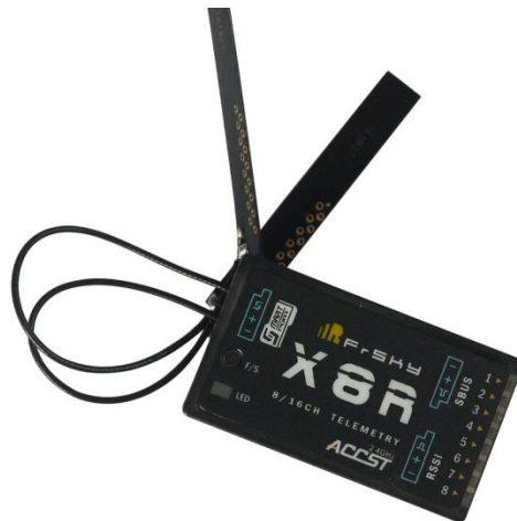
Figura 3.9 Receptor FrSky X8R
