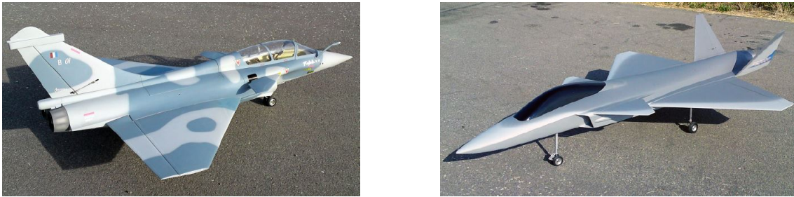
Figure 1.3: Two of the sub-scale research aircraft and concept demonstrators available at Linköping University. Left: Dassault Rafale fighter test-bed. Right: Generic Future Fighter. Courtesy of Linköpings University.
