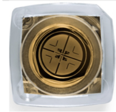
Figura 17. Célula SMRT conteniendo 150000 ZMW (zero-mode waveguide) (Pacific Bioscience, 2009)
