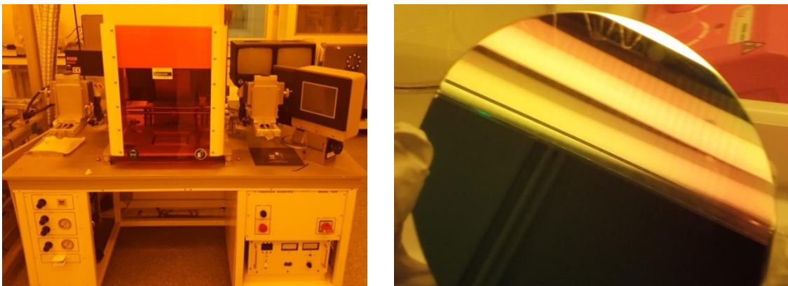
Fig. 14. Mask aligner and exposer (left) and wafer with developed photoresist (right)
