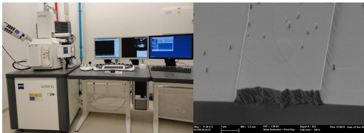
Fig. 17. Picture of the Scanning Electron Microscope (left) and silicon nitride waveguide obtained after the photolithography process (right).
