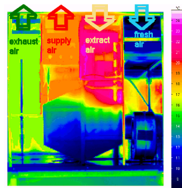
Figure 16: Counterflow heat recovery system
