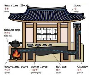
Figure 6: Ondol system in Korean traditional architecture.
