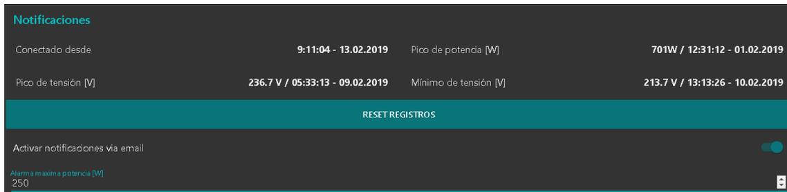
The screenshot shows a 'Notificaciones' (Notifications) section with a table of power and voltage records. The table has two columns for power and two for voltage. Below the table is a 'RESET REGISTROS' button and a toggle for email notifications. At the bottom, there is a 'Alarma máxima potencia [W]' field set to 250.
