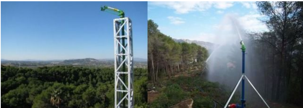
Figure 14. On the left is a column of lattice-type emission and on the right a column of braced emission, both created by the company SIDEINFO® for the prevention of forest fires. Source: official website of SIDEINFO®.
