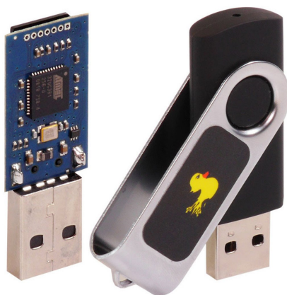
Figura 5.2: USB Rubber Ducky de Hak5.
