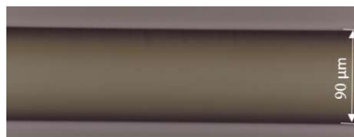
Figure 2.5.1. The commercial graded index multimode perfluorinated fiber after etching under microscope.
