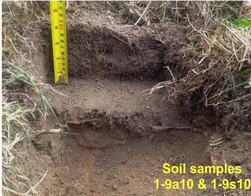
Figure 8: Typical preparations for soil sample collection at 10 cm depth. Sample ID clarification (exemplary case 1-9a10 and 1-9s10): first number stands for sampling period (1 – autumn), second number denotes subplot (9), the letters a and s are for sampling point and mixed sample identification respectively and the third letter (10) marks the depth of sampling. Note how dry the soil profiles were during the first sampling.
