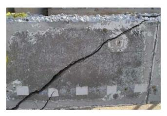
Figure 4. A typical shear/bond failure (specimen NSC-3D)
