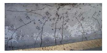
Figure 3. A typical flexural failure (specimen NSC-2L)
