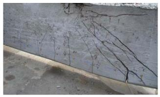
Figure 5. A typical bond failure (specimen HSS-4L)
