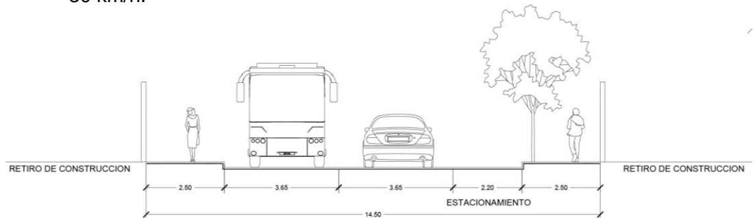
COLECTORA A 14.50m.
