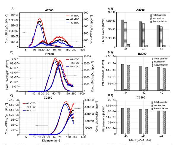
Figure 8. Influence of SoE2 over particle size distributions and PN emissions at each operation mode.
