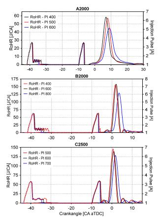
Figure 3. Effect of IP over RoHR at each operation mode.
