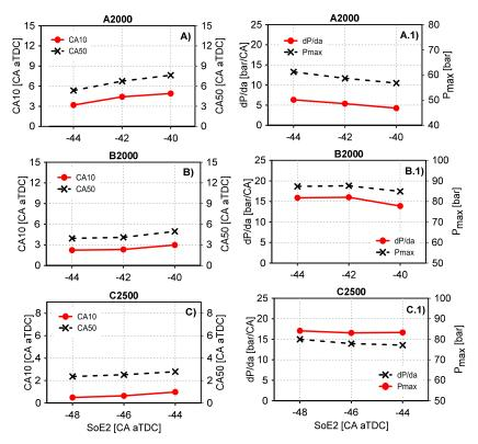
Figure 7. Effect of SoE2 over the  $dP/d\alpha_{max}$ ,  $P_{max}$ , CA10 and CA50 at each operation mode.
