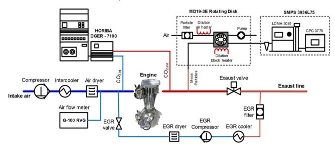
Figure 1. Experimental set-up for the evaluation of PN emissions and PSD in steady-state operating conditions.
