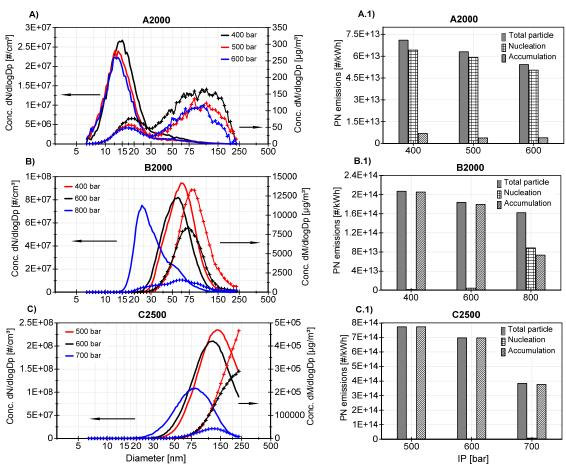
Figure 5. Influence of IP over particle size distributions and PN emissions at each operation mode.
