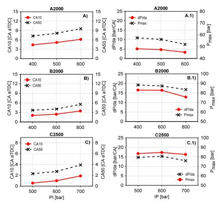
Figure 4. Effect of IP over the dP/d $\alpha_{max}$ ,  $P_{max}$ , CA10 and CA50 at each operation mode.
