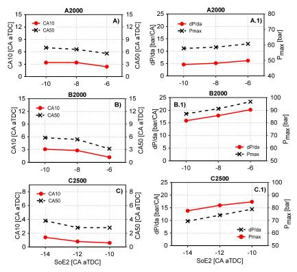
Figure 10. Effect of SoE3 over the dP/d $\alpha_{max}$ ,  $P_{max}$ , CA10 and CA50 at each operation mode.
