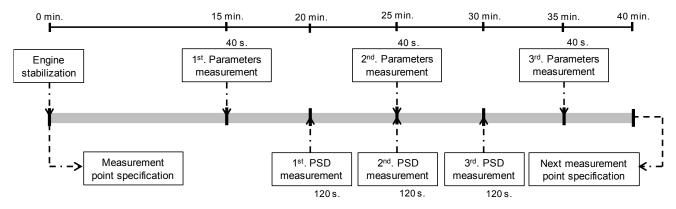
Figure 2. Methodology applied for PSD and different parameters (EGR rate, air mass and fuel mass) measurement at each steady-state operating point.
