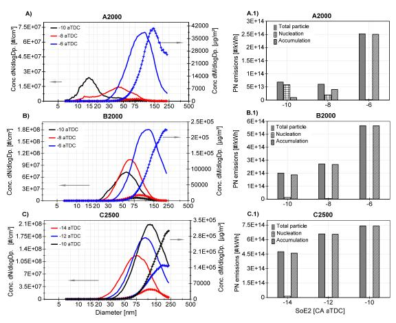
Figure 11. Influence of SoE3 over particle size distributions and PN emissions at each operation mode
