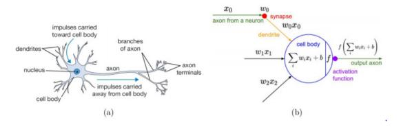
Figure 2.3: Representation of a biological neuron (a) and its mathematical model (b).
