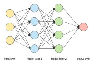
Figure 2.4: Architecture of a Neural Network.
