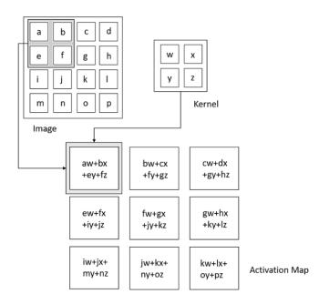
Figure 2.5: Representation of a Convolutional Layer operation.
