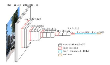
Figure 2.8: Representation of the VGG16 network architecture.
