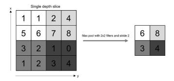
Figure 2.6: Representation of a Pooling Layer operation.
