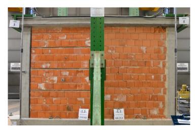
Figure 18. Behaviour of RJ and MJ walls during in plane test at 1.2% drift (INSYSME, 2013).
