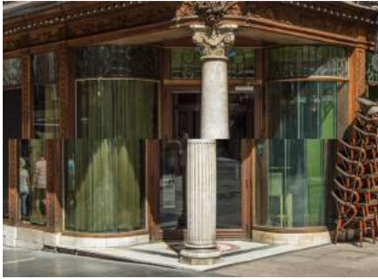
Fig. 133. Álvaro Salido: Split focusing system of Sankyo ES-44 XL super-8 camera. The split column seen through the camera lens is out of focus.
