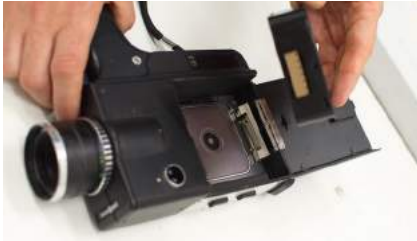
Fig. 129. Super-8 cartridge about to be inserted into the camera.
