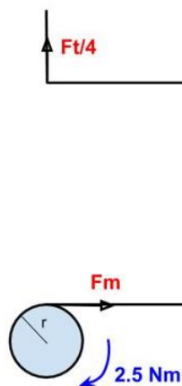
Figure 30. Schema of the momentum and force applied by the stepper motor on one cable and one pulley.
