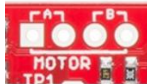
Figure 35. Top left corner of the EasyDriver, where the stepper motor is connected.
