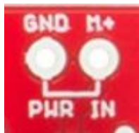
Figure 37. Top right corner of the EasyDriver where the power source is connected.
