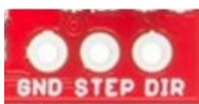
Figure 39. Bottom right corner of the EasyDriver where the Arduino is connected.
