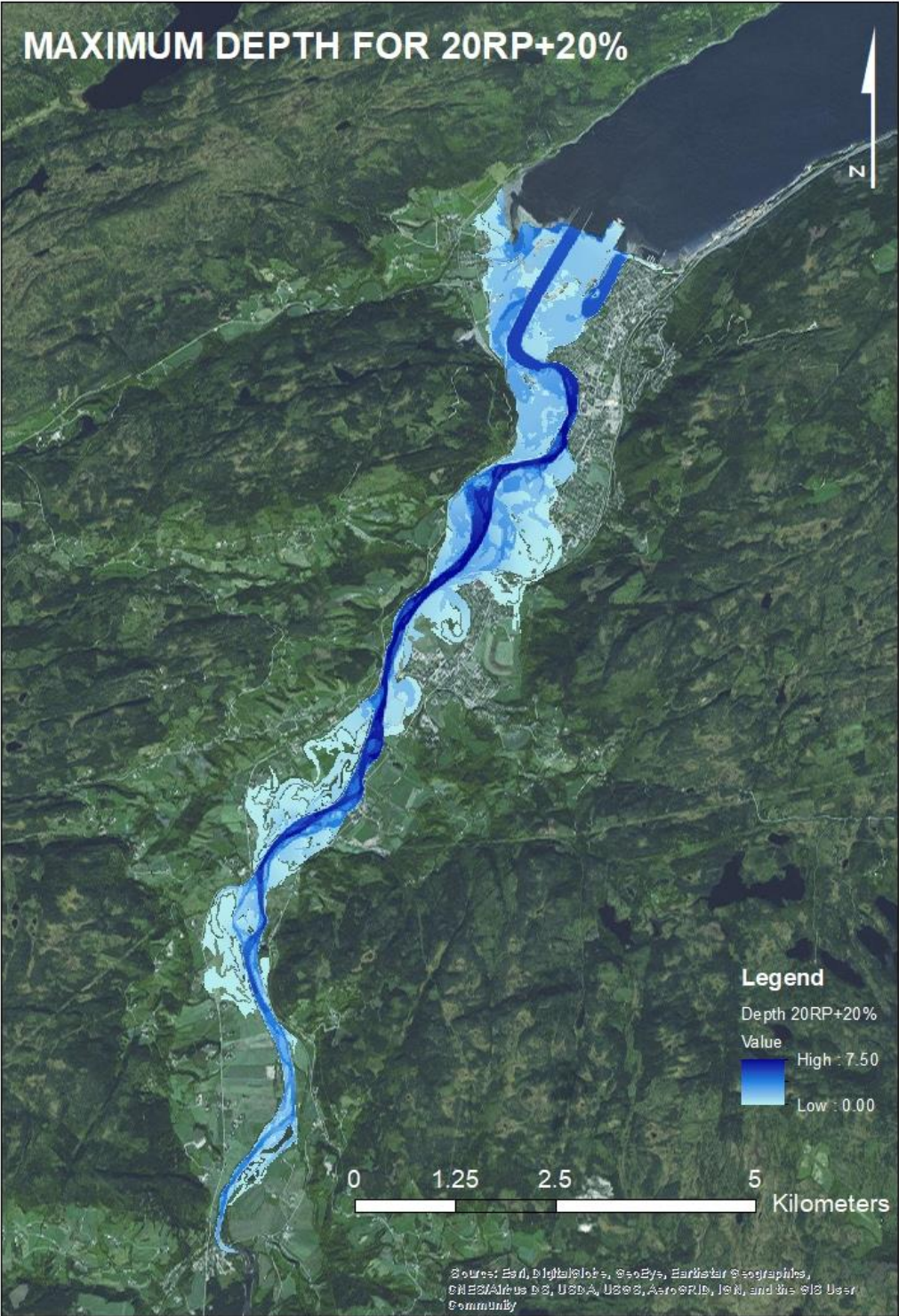
Figure 18: Layer of depth obtained by simulate the hydraulic model for 20 years RP+ 20% of peak flow
