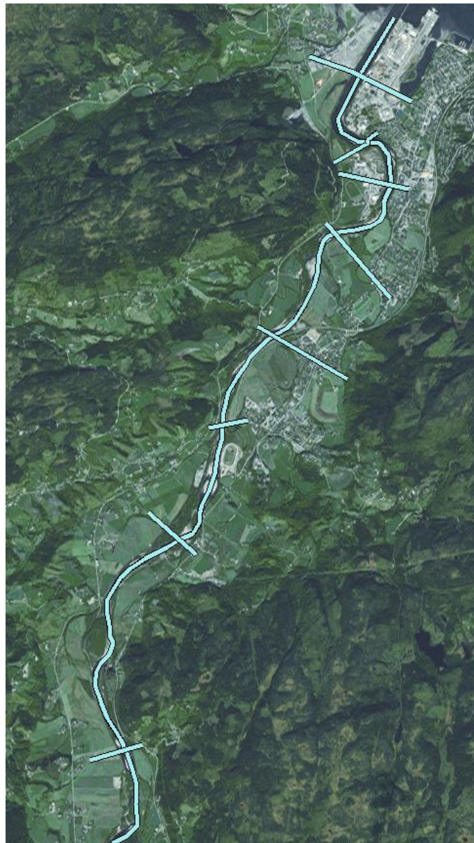
Figure 26: Cross Sections for flood variables study
