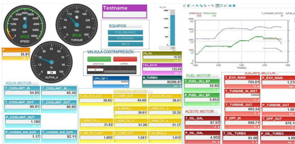
FIGURE 17: PUMA's control screen.
