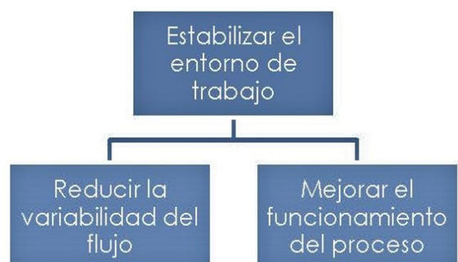
Fig.7: Los principios básicos de Last Planner System® (Fuente: Ballard y Howell, 1994) / The basic principles of Last Planner System® (Source: Ballard and Howell, 1994)
