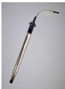
Figure 3: Reference Ag/AgCl electrode
